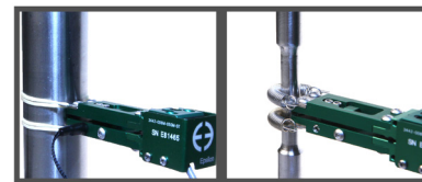
Rubber band and spring attachment options included with Models 3442 and 3542
