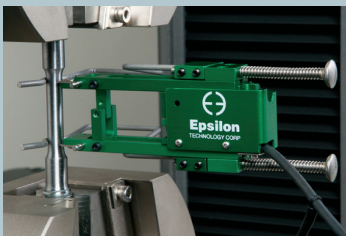
Model 3542 with 25 mm gauge length
