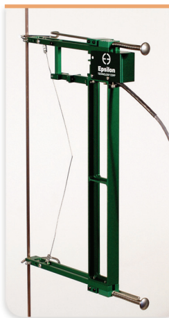
Model 3542L with 8 inch gauge length and +0.5 inch/-0.25 inch measuring range
