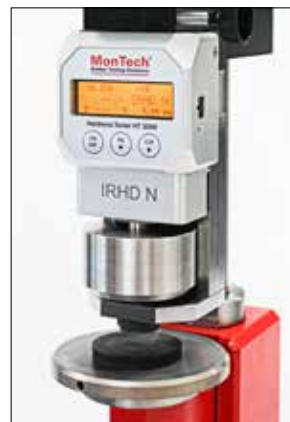
IRHD Normal measurement on parts
