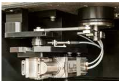
Rheometer brushless DC drive upgrade
