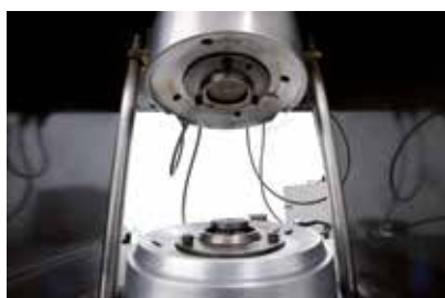
Die upgrades including precision heaters and probes
