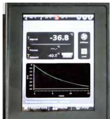
Sample temperature recording by optional immersion probe
