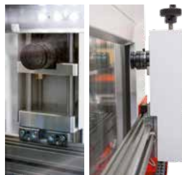
CCD Camera system for crack-growth measurement
